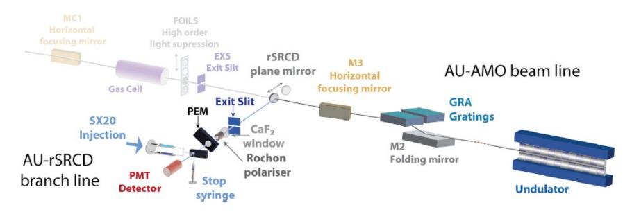
Two liquid samples are mixed, and the reaction is followed on *ms* scale
