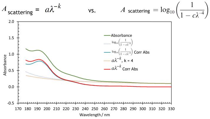
Fit to 330-310 data: same curve above 230 nm, but not below Absorbance difference at 205 nm is about 5%
