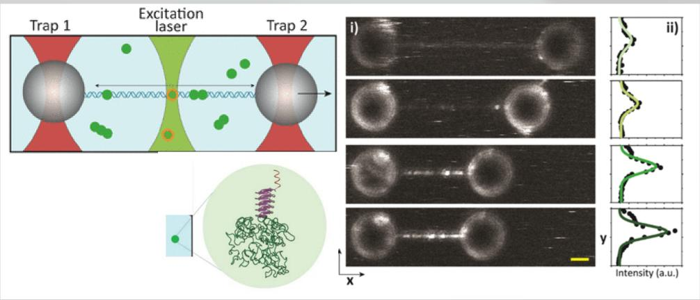
Optical tweezers combined with fluorescence confocal microscopy reveal protein binding and compaction into the virus capsid.
