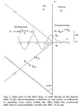
Fig. 2. Side view of the IRE (Fig. 1) with details of the electric field of the electromagnetic radiation at one point of reflection. A standing wave exists within the IRE while the evanescent field decays exponentially outside the IRE. Z in μm.
