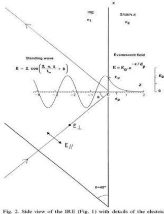
g. 2. Side view of the IRE (Fig. 1) with details of the electric ld of the electromagnetic radiation at one point of reflection. ding wave exists within the IRE while the evanescen cays exponentially outside the IRE. Z in ur
