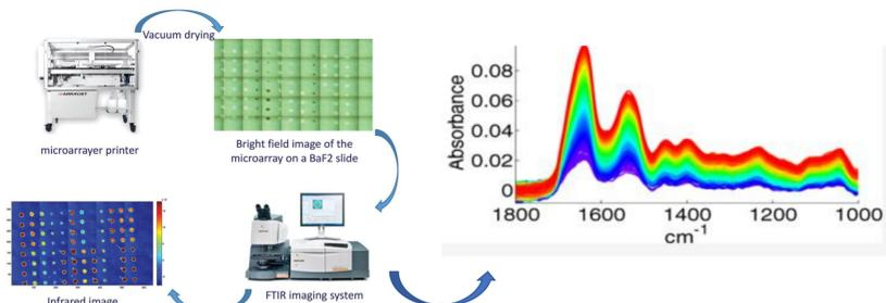
Each spot contains 1 ng of proteins (in 100 pL). Each spot has a diameter of ~80 μm. Each protein is printed in four replicates and gives > 200 high quality spectra that are averaged.
