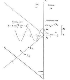
Fig. 2. Side view of the IRE (Fig. 1) with details of the electric field of the electromagnetic radiation at one point of reflection. A standing wave exists within the IRE while the evanescent field decays exponentially outside the IRE. Z in μm.
